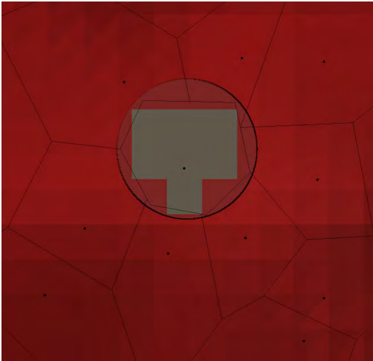
Figure 2-3: Example pier insertion and computational mesh
