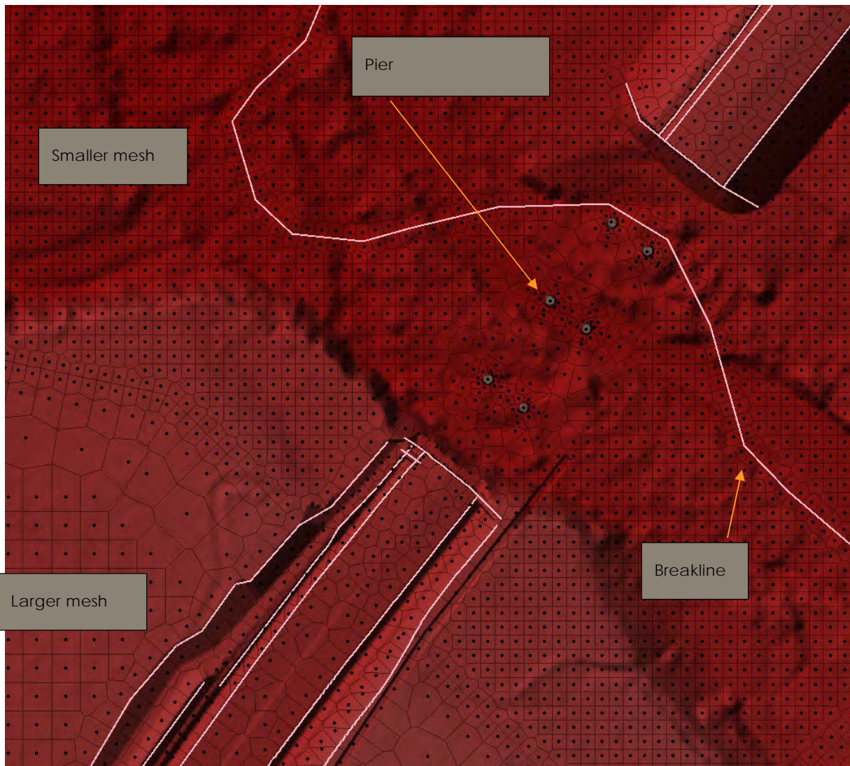
Figure 2-2: Example (Waikawa) 2D bridge with mesh and breaklines
