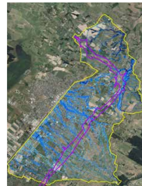
Baseline maximum modelled depths, showing 1:100 flood event in 2030 (North) [Technical Assessment - Hydrology and Flooding]
