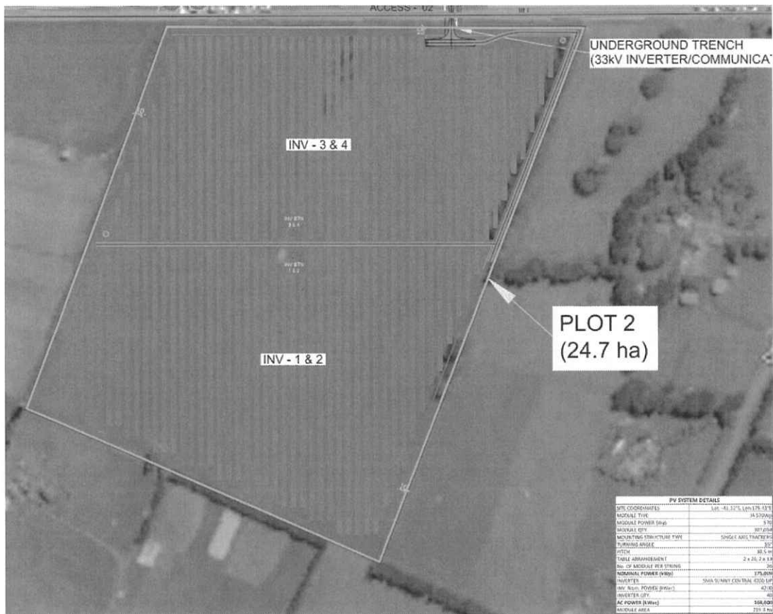
Figure 7: Array layout view 1
